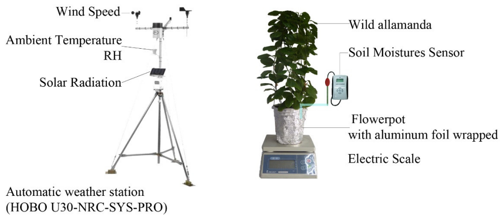
Figure 1. Diagram of potted transpiration measurement
